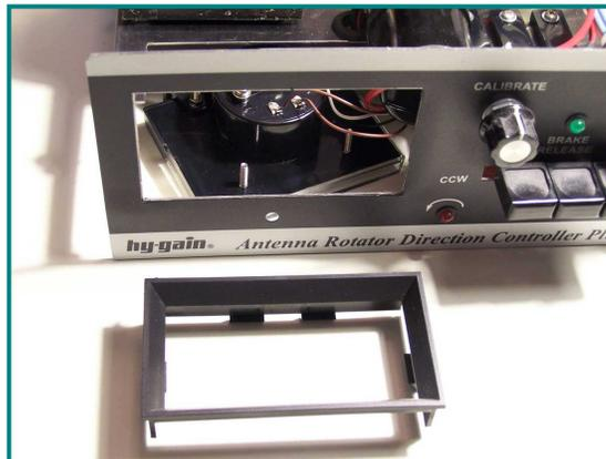
11. You have several options of removing the top part of the enclosure to allow the LEDs to shine through onto the top of the meter. Example: drilling 3 holes with the proper spacing. Then re-insert the enclosure back into the front panel and reinstall the meter.
