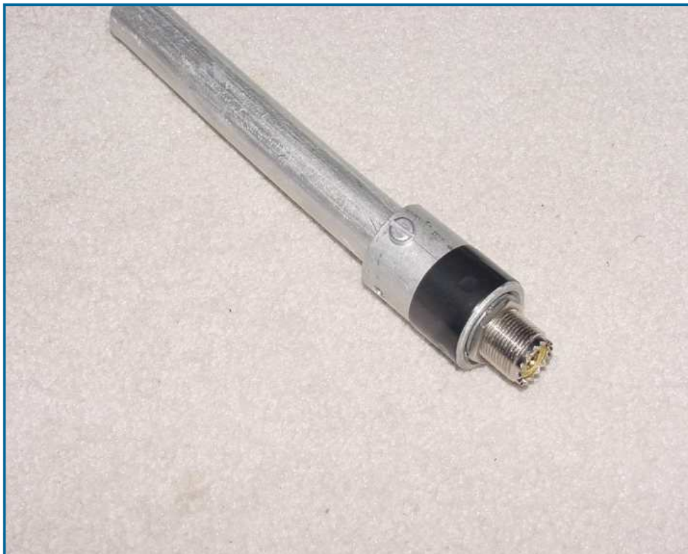
Figure 4 - Completion merely requires threading on the Aluminum shield Coupler and securing with screws.
