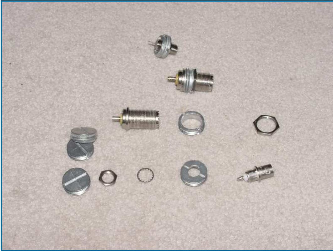
Figure 1: Threaded aluminum plugs of the kind sold to seal off unused holes in outdoor electrical junction boxes are drilled to accept a variety of RF connectors.
