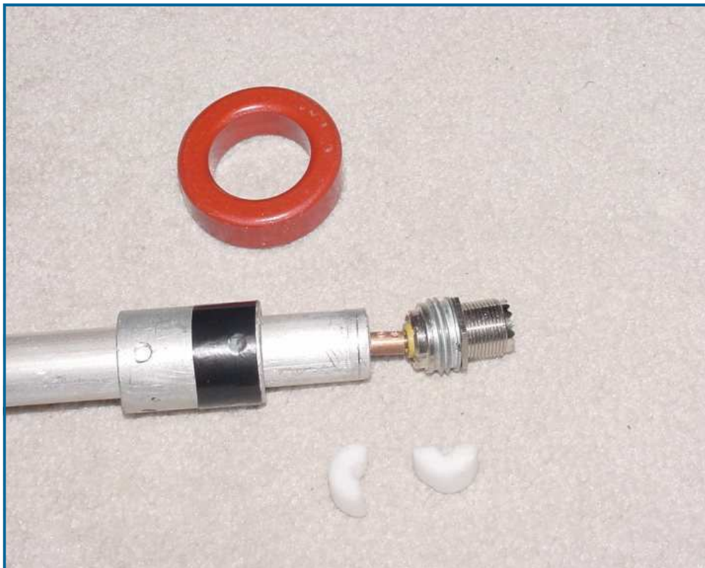
Figure2 - Here the prepared connector plug center pin is being soldered to the cable center pin via a 1/2" length of 1/4" copper tubing ( typical as used in icemaker installations).
